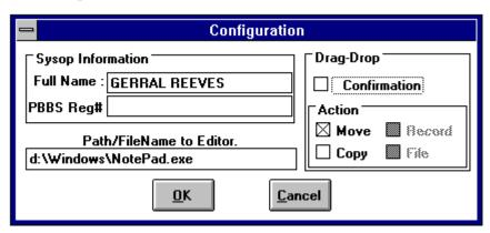
This is the Configure window. First set the <u>Path/FileName</u> for your ASCII editor. Then set the Confirmation for the drag-drop, set it to Checked, if you want a confirm dialog box when you drag-drop files. next selext <u>MOVE</u> or <u>COPY</u> for the drag-drop operations. If you select copy, then you must also select, File and/or Record, this tells PBBSFMGR what to copy. The Sysop Name is optional.
